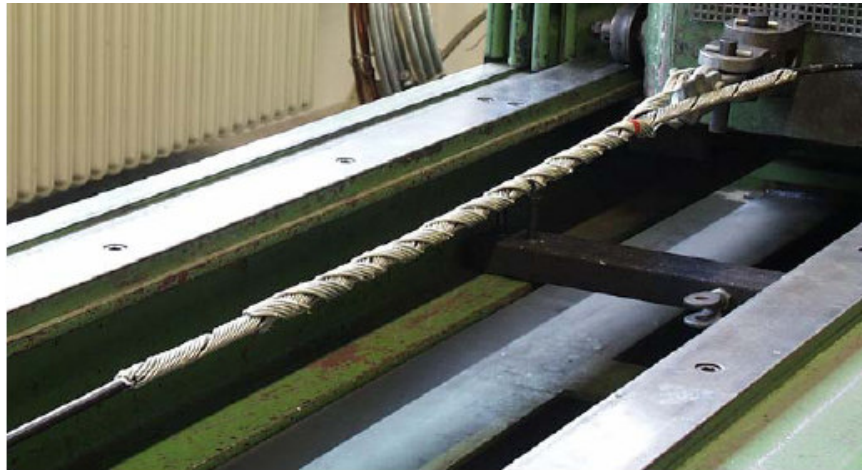
Figure 3. Testing for cable Grip
